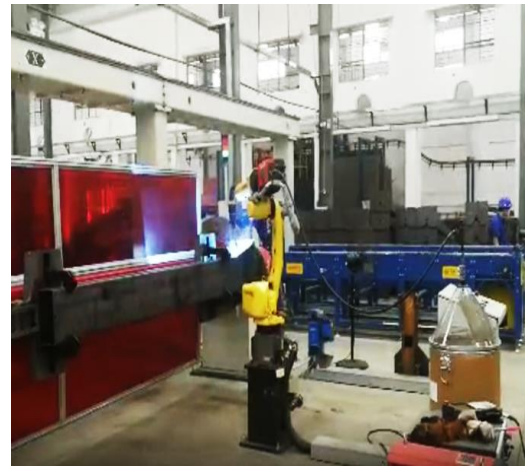
Figure 1 Robot welding of HAPP columns http://happ.com.au/pub/vid/columnwelding.mp4
